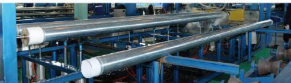
Steel Pipe of Lining Plastic Production Line
