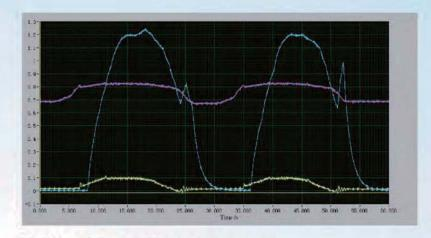
Quickly open to release the over-pressure Slowly close to prevent a second surge damage
