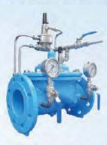
The Model 1340B Burst Control Valve is a hydraulically operated, diaphragm actuated control valve. It shuts off and locks drip tight upon sensing flow in excess of setting, until it is manually reset. As long as flow is lower than the setting, the valve remains fully open, minimizing head loss.
