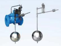
The Model 1310B Float control Valve is a non-modulating valve that accurately controls the liquid level in tanks. This valve is designed to open fully when the liquid level reaches a preset low point, and close drip-tight when the level reaches a preset high point.
