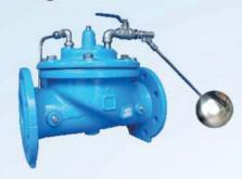
The Model 1310 Float Valve is a modulating valve that accurately controls the liquid level in tanks. This valve is designed to open fully when the liquid level reaches a preset low point, and close drip-tight when the level reaches a preset high point. The float pilot is remotely installed inside of reservoir.
