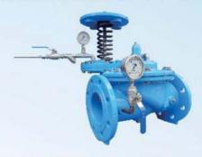
The Model 1310A Altitude Valve controls the high water level in reservoirs without the need for floats or other devices. It remains fully open until the shut-off level is reached.
