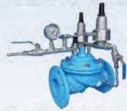
The Model 1355 Surge Anticipating Valve is indispensable for protecting pumps, pumping equipment and all applicable pipelines from dangerous pressure surges caused by rapid changes of flow velocity within a pipeline.
