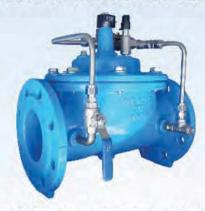
The Model 1360 Solenoid Control Valve is an on-off control valve that either opens or closes upon receiving an electrical signal to the solenoid pilot control. This valve consists of a main valve and a two-way solenoid valve that alternately applies pressure to or relieves pressure from the diaphragm chamber of the main valve. It is furnished either normally open (energized solenoid to close) or normally closed (energized solenoid to open).
