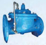
The Model 1330 Check Valve is a hydraulically operated No-Slam Check Valve. This valve opens when the pressure at the inlet exceeds the discharge pressure. A gradual rate of opening prevents sudden opening surges. When a pressure reversal occurs the higher downstream pressure is applied to the cover chamber through the control tube lines, and the valve closes drip tight. This valve is ideally suited for use where a positive shutoff is required. The rubber disc assures tight sealing.
