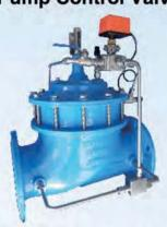
The Model 1370 Pump Control Valve is a pilot operated valve designed for installation on the discharge of booster pumps to eliminate pipeline surges caused by the starting and stopping of the pump.
