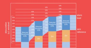
TrueAlarm sensors are engineered to maintain their present levels of sensitivity. As dirt accumulates, the sensors self-adjust, notifying operators of Almost Dirty, Dirty and Excessively Dirty conditions long before they trigger a nuisance alarm. This lets you schedule maintenance on both Dirty and Almost-Dirty sensors at the same time, minimising your facility costs.
